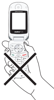
INCORRECT FINGER POSITION
