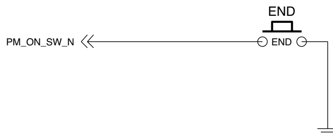
Figure 1.20 END Keypad Circuit
