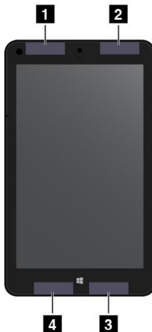
Figure 5. Location of the UltraConnect wireless antennas
